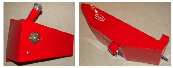
3.5 Jedi Slipper Tank installation – Support the tank from underneath, then position it onto the hull and temporarily fit the support strap. Mark the tank brackets with a felt pen at the airframe's tank mounting hole locations. The length of the rear mounting brackets of the Jedi slipper tank is designed to make any existing plastic spacer blocks
