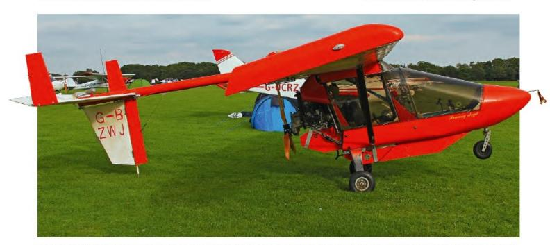
Because of the nature of the design, the Shadow series of aircraft rest on their tail when the pilot's weight is removed; you can see that it would be easy to inadvertently impart quite large loads through the fin post into the fuselage boom and it's definitely worth taking this into account when pull starting the engine. (Photo: Richard Hamblyn)
