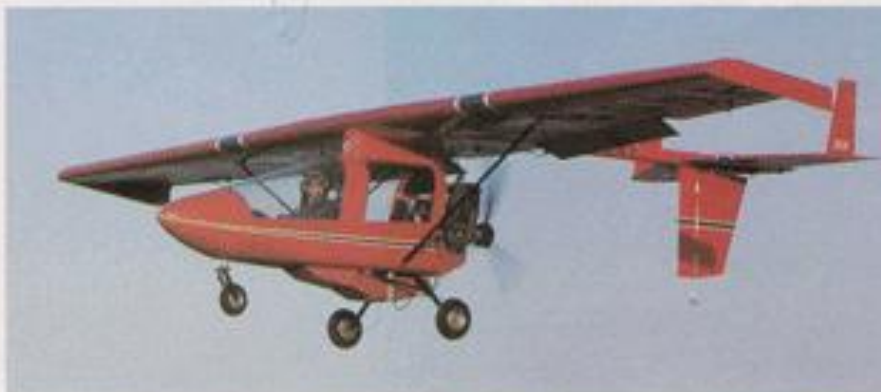
Triple-fin arrangement may not be the most elegant, but it works well at all speeds. Dave Cook parks his Streak and the trailer he occasionally transports it on a cricket pitch that is also his 'aerodrome'. The Rotax 532 is twin-cylinder, water-cooled; starting is by toggle, with an electric starter an option.
